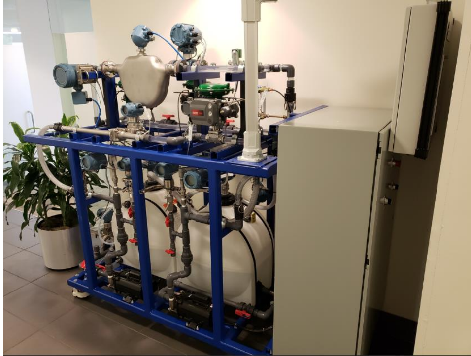
Figure 2. Representative example of a DeltaV process skid used in industrial automation environments. This image illustrates the type of modular, small-scale process hardware under consideration for developing a virtualized control room research environment focused on human-machine interface (HMI) evaluation and operator performance studies.
